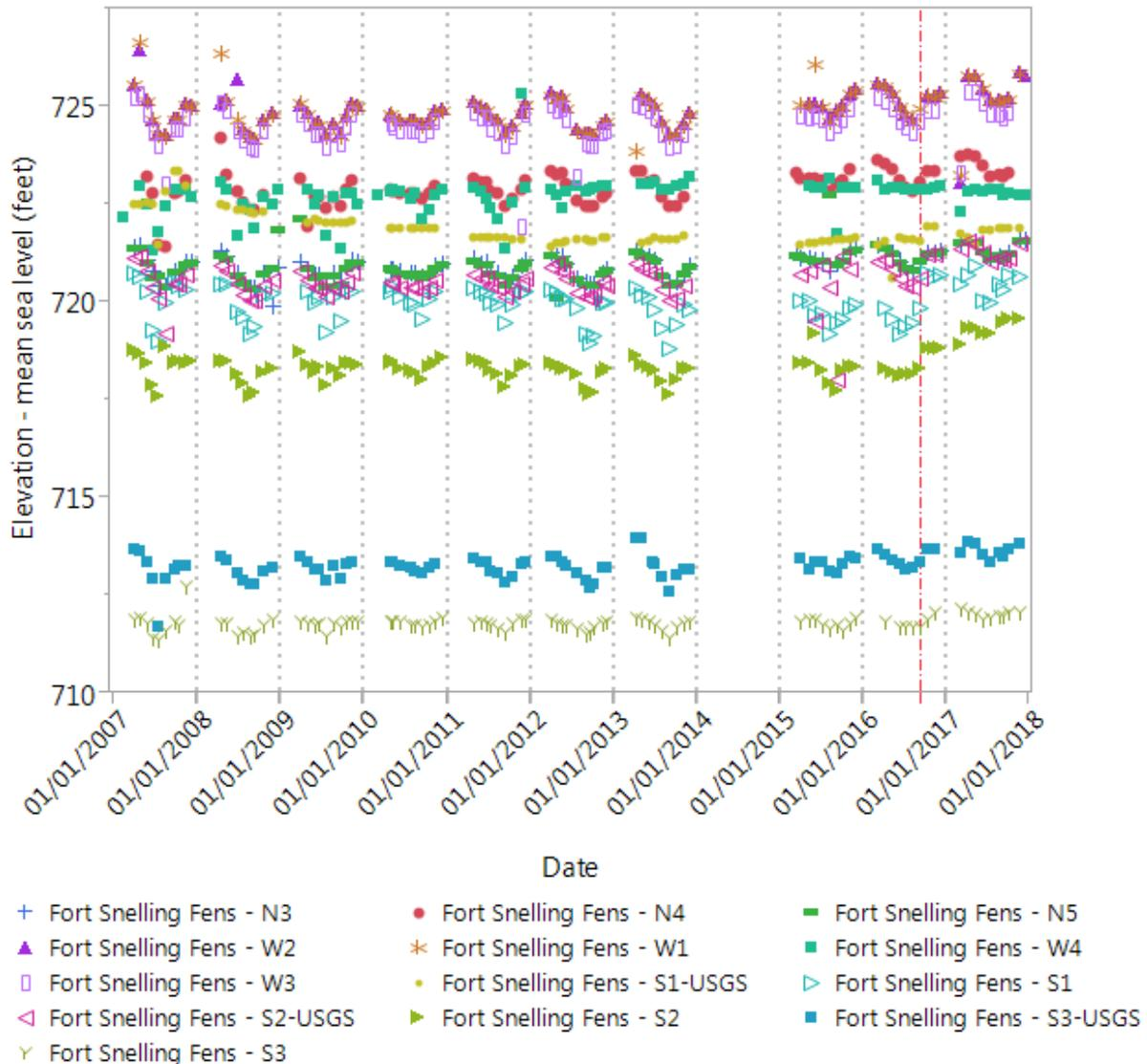
**Figure 3.** Water level elevation for the Fort Snelling fen wells. At well S3-USGS, when the water was overflowing, the elevation of the top of the pipe (Historical - 713.97 and 2016 – 714.18) was recorded. See individual well graphs in Appendix 3.
