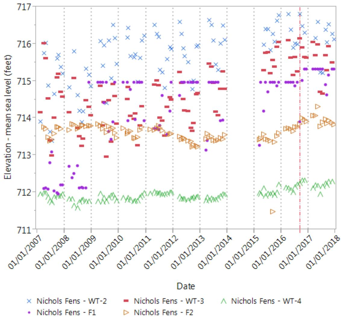
**Figure 6.** Water level elevation for the Nichols Fen wells (set 3 of 3). At well F1, the water was often overflowing and the elevation of the top of the pipe (Historical - 714.97 and 2016 – 715.32) was recorded. See individual well graphs in Appendix 3.
