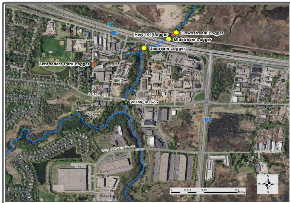
Figure 2. Location of temperature loggers and WOMP station. The loggers added in 2018 are represented by the orange triangles. Thermal water data at the WOMP station is collected with MCES monitoring equipment.
