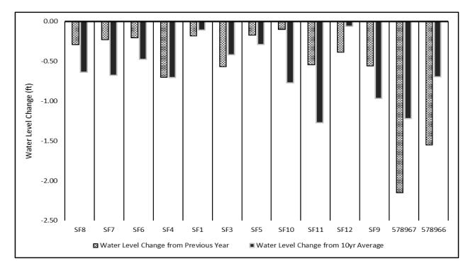
**Figure 21.** The water level changes at each Savage Fen well when compared with the previous year and the 10yr average depth to water. Average 2021 depth to water levels were used to compare with average 2020 values and 10yr historical average.
