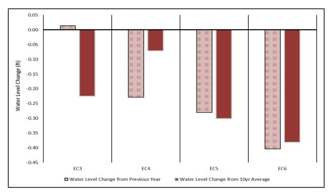
**Figure 26.** The water level changes at each Eagle Creek well when compared with the previous year and the 10yr average depth to water. Average of all 2021 DTW measurements collected were used to compare with average 2020 values and 10yr historical averages.
