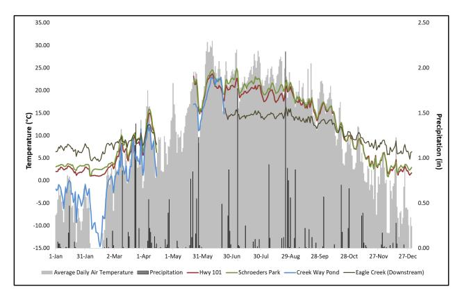
Figure 6. Pond outlet loggers 2021 average daily water temperatures. The Eagle Creek downstream logger is shown for reference.
