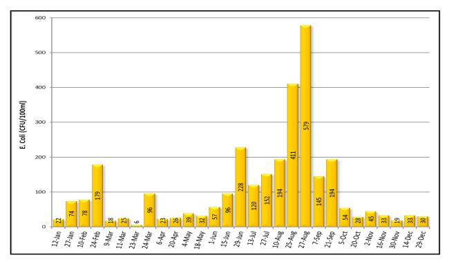
**Figure 12.** *E. coli* samples (2021). *E. coli* state standard for class 2A waters is not to exceed 126 organisms/100 ml as a geometric mean of not less than 5 samples representative of conditions within any calendar month. Nor shall more than 10% of all samples taken during any calendar month individually exceed 1,260 organisms per 100 ml. The standard applies only between April 1 and October 31.
