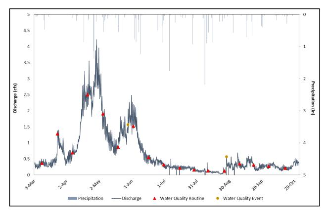
Figure 14. Dean Lake Inlet continuous 15min discharge data, precipitation, and water quality samples collected in 2021.
