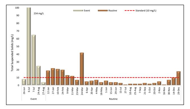
**Figure 10.** Total Suspended Solids (2021). State Standard for Class 2A Waters = 10 mg/L (indicated by the red dashed line and the shaded areas in the graph) with no more than 10% exceedance between 1 April and 30 September.
