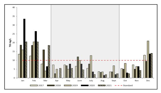
**Figure 11.** Total suspended solid monthly average over the last 5 years for non-event samples. The state standard is 10mg/L indicated by the dashed red line. No more than 10% exceedance shall occur between 1 April and 30 September (shaded area).
