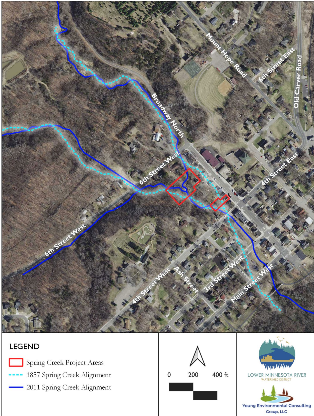
Figure 8. Change in Spring Creek Alignment
