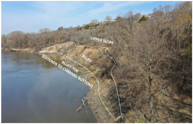
Figure 2: Drone image with schematic lines showing site descriptor terminology used in this report.
