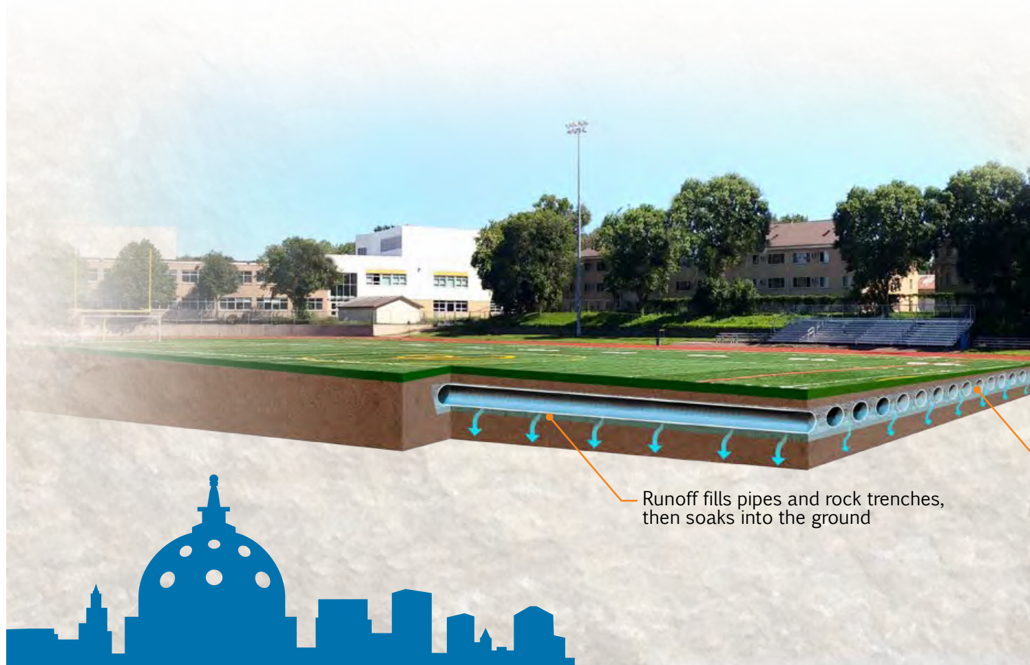
Polluted stormwater runoff enters infiltration gallery from storm sewer on Rose Avenue.
