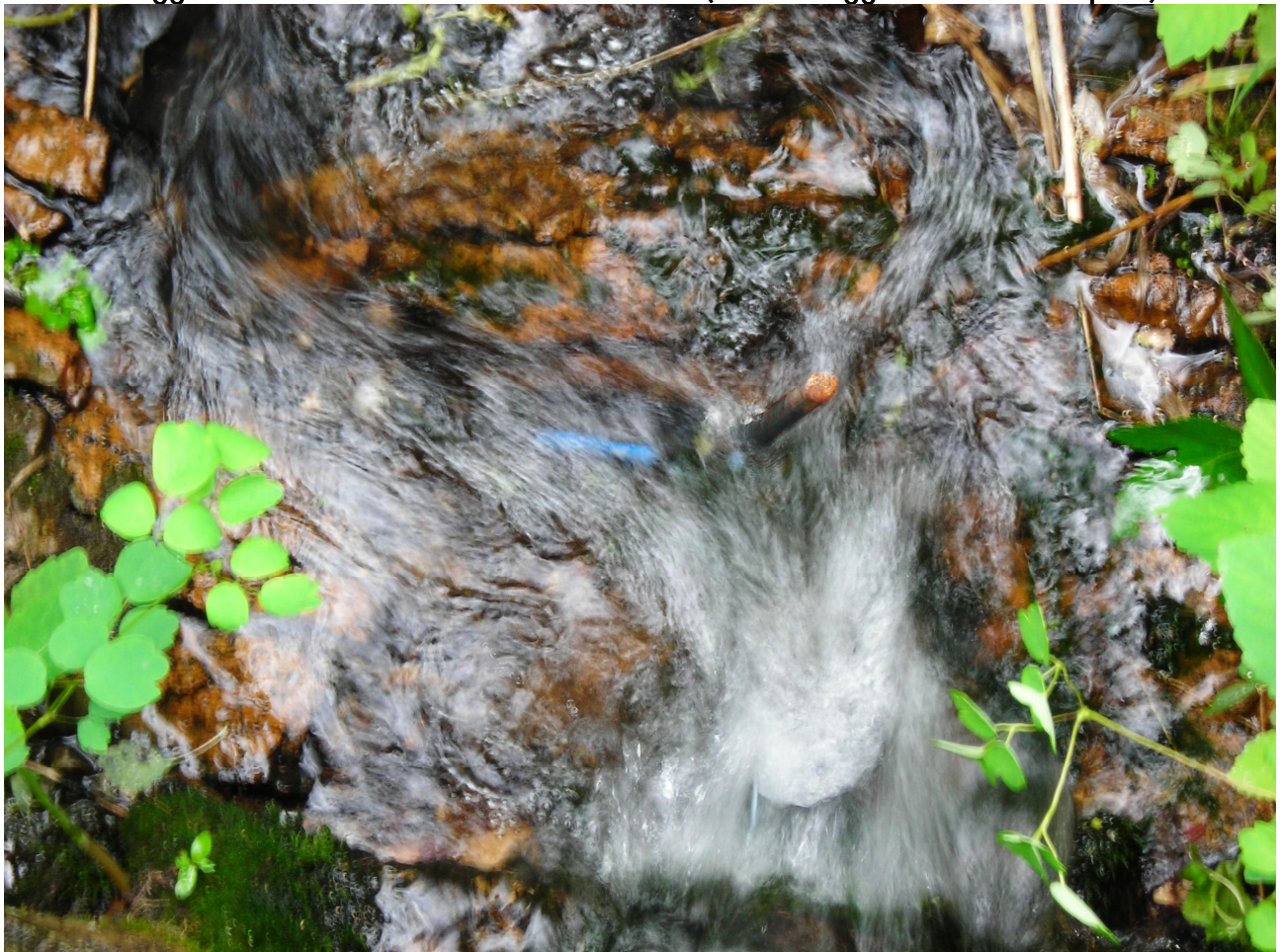
Logger installed at the outlet of the culvert (view of logger in main flow path)
