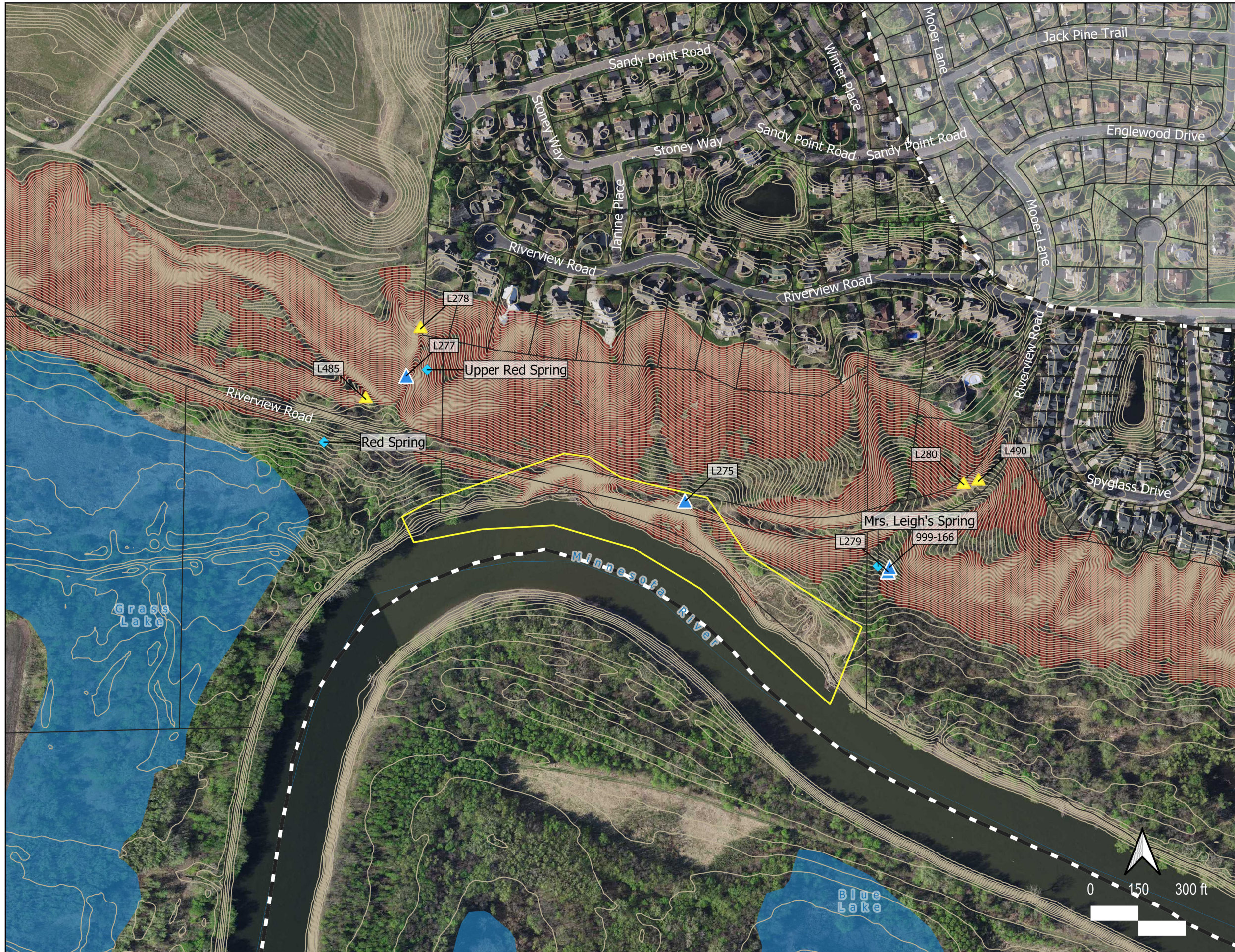
Figure 5: Area 3 Groundwater Observations
