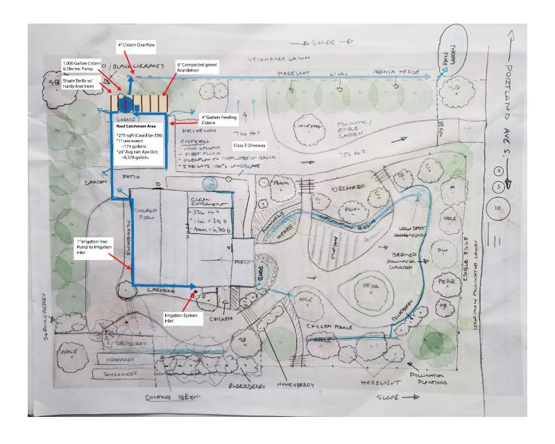
Imagine the same setup shown below on the North side of the garage. The overflow will be directed into a low laying area near the cistern where water will infiltrate and irrigate the water loving plantings nearby. If the overflow is very large, the water will them slowly travel ~150' through grass, infiltrating and irrigating fruiting shrubs along the way before it ever enters the street. \*Foundation will be 6" of compacted gravel after excavation of topsoil.
