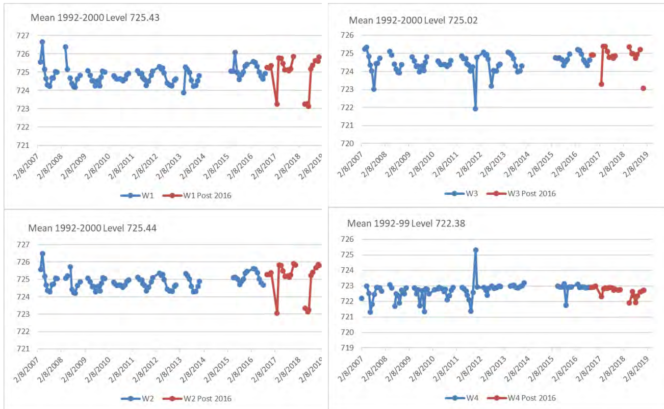
Graph 4-5. Groundwater Levels in Gun Club Lake South Wells Designated “W” (From left to right, top to bottom: 482157, 482154, 591979, 591980)
