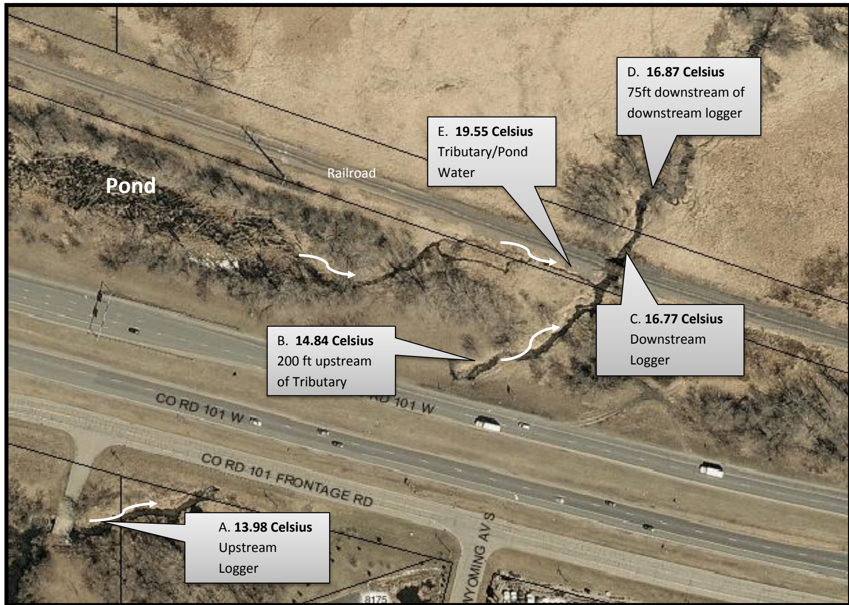
Figure 3. Investigative Temperature Monitoring During Rain Event. White arrows indicate flow direction. Callouts indicate temperature values taken at approximately 4:00pm on August 19, 2009 during a 2" rain event. Notice temperature increase between (B) and (C). Tributary (E), which comes from the pond, is contributing warmer water than the direct contribution from Highway 101 (estimated that 5–10 cfs water coming from tributary during time of measurement).
