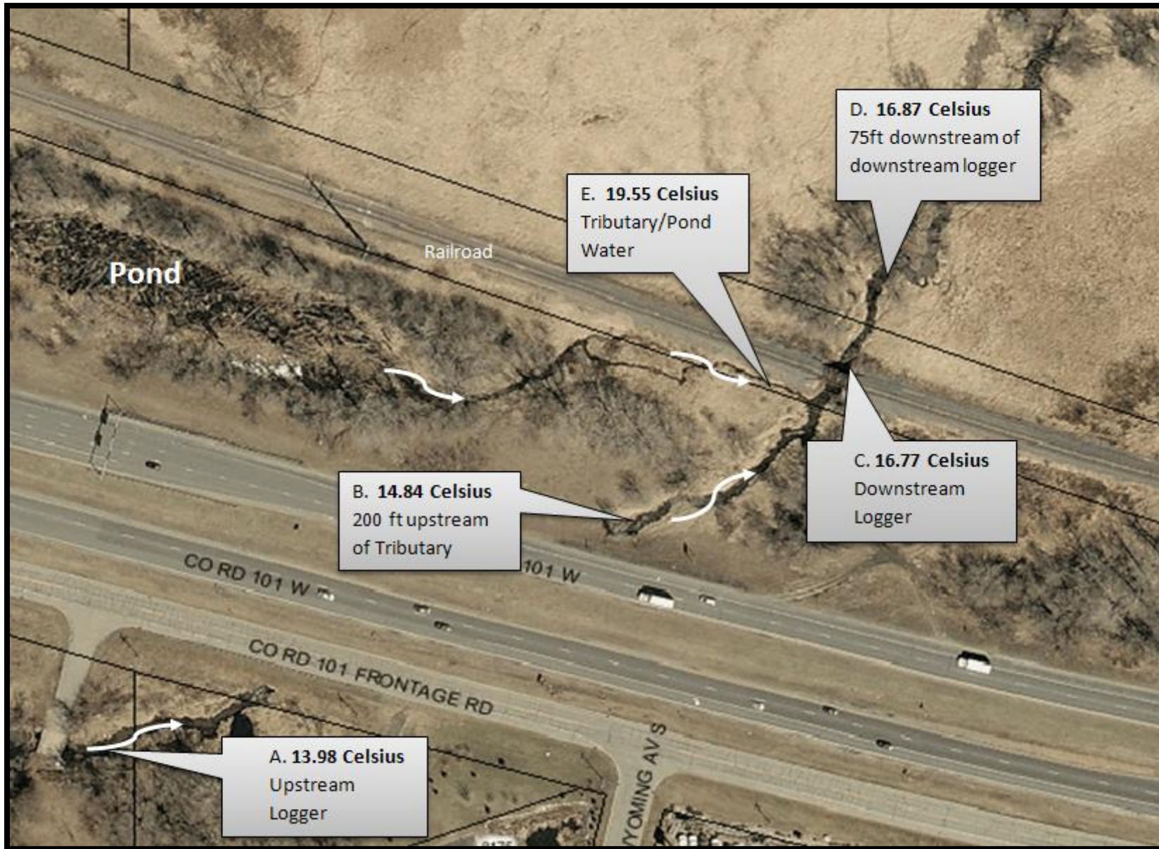
Figure 4. Investigative Temperature Monitoring During Rain Event. White arrows indicate flow direction. Callouts indicate temperature values taken at approximately 4:00pm on August 19, 2009 during a 2" rain event. Notice temperature increase between (B) and (C). Tributary (E), which comes from the pond, is contributing warmer water than the direct contribution from Highway 101 (estimated that 5–10 cfs water coming from tributary during time of measurement).
